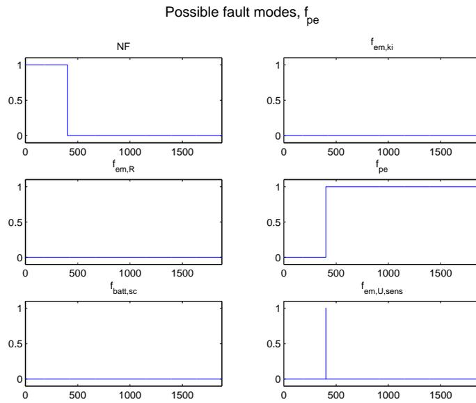
Figure 4.16: Possible fault modes when  $k_{pe}$  is halved at 400 seconds. This fault is also detected and isolated in 3 seconds after it occurs.
