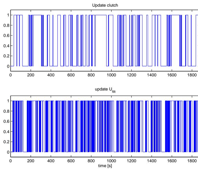
Figure 4.48: The tests are updated when all conditions required for the actual test are fulfilled. Test 1 is for example valid all the times, but test 6 only when both the clutch is engaged and  $|U_{filt}| > 1$  V. When different limitations are used are shown in this figure.
