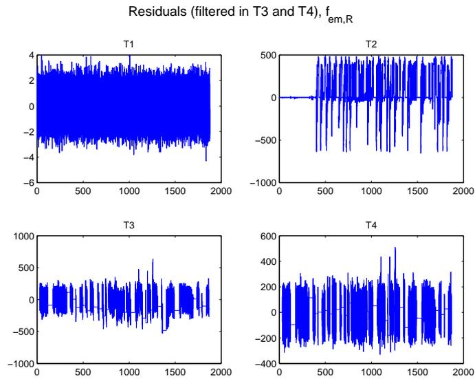
Figure 4.34: The residuals when  $R_{em}$  is halved at 400 seconds. It is obvious that the residual in test 2 changes characteristics after 400 seconds when the fault is induced, but it is not in the residual used in test 3.
