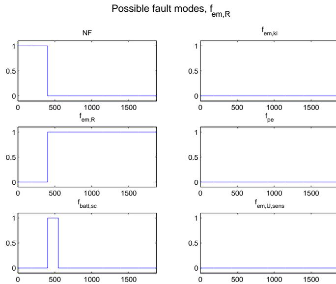
Figure 4.33: The possible faults when  $R_{em}$  is halved at 400 seconds. The fault is detected after a few seconds, but it takes about 150 seconds to isolate the fault since this is the time it takes for test 3 to react.
