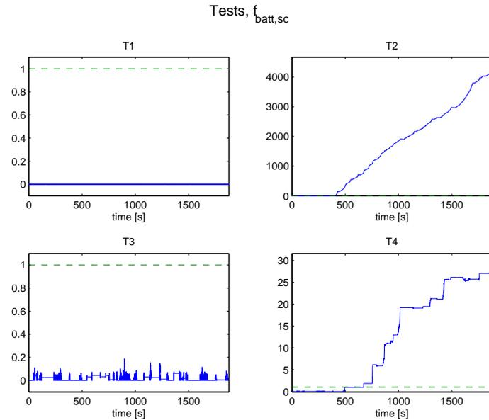
Figure 4.41: Normalized test before threshold when  $k_{sc}$  is halved at 400 seconds. Compared to the other faults test 4 reacts on, the magnitude of the test quantity is larger. It has neither the trend of decreasing at the end of the simulation as is the case when  $f_{em,ki}$  is detected in Figure 4.32.
