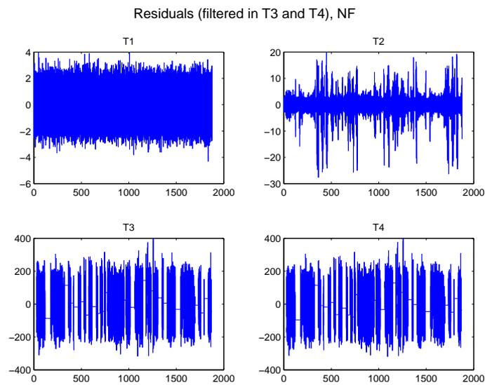
Figure 4.27: The residuals in the fault free case. The residuals used in tests 3 and 4 are not updated at all times. This depends on several conditions explained in each test above. Note that the tests are not being updated the first 10 seconds after the residuals have been valid again.
