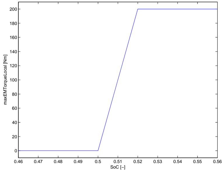
Figure 3.1: The maximum torque the electric motor is allowed to deliver as a function of  $SoC$ .
