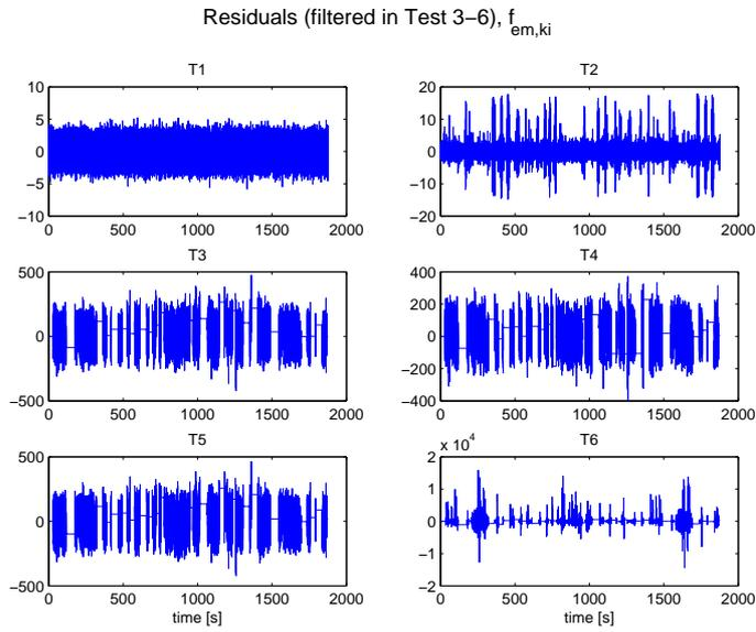
Figure 4.50: The residuals when  $k_i$  is halved at 400 seconds. Note that even when the residuals are calculated it is not sure that the test quantity is updated.
