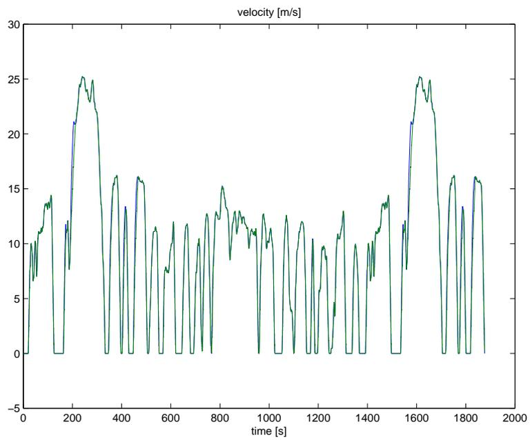
Figure 3.3: The velocity of the truck when it tries to follow the drive cycle, FTP75.
