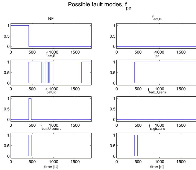
Figure 4.55: Possible fault modes when  $k_{pe}$  is halved at 400 seconds. The fault is detected fast and full isolability is achieved for some time.
