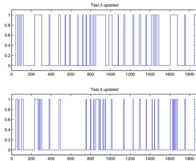
Figure 4.29: This figure includes information about when the tests are updated. When the signal is 1 the test is updated and the conditions for when the tests are updated are stated in each test above. This signal is 0 during the first 10 seconds after the conditions set up in the tests for the system to be valid are fulfilled.
