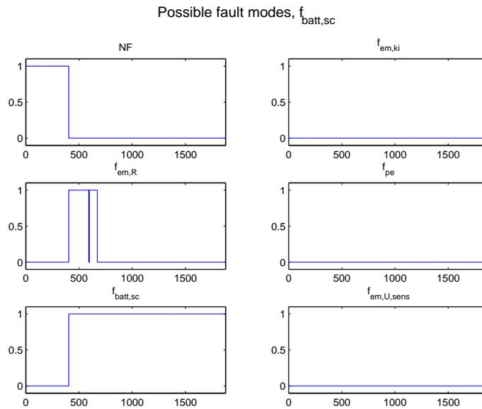
Figure 4.39: Possible fault modes when a short circuit in the battery occurs at 400 seconds resulting in that only half of the cells are only used after this time. The fault is detected in a few seconds after it is induced in the model, but It takes almost 300 seconds to achieve isolability of the fault since this is the time it takes for test 4 to react.
