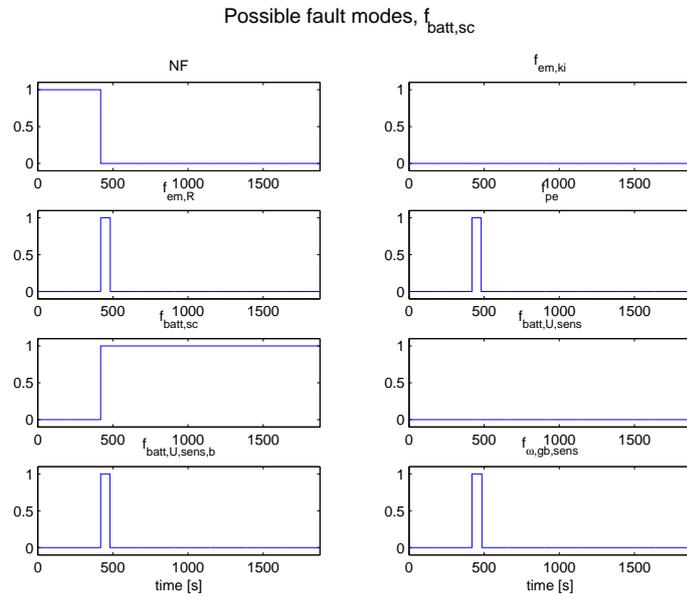
Figure 4.58: The possible fault modes when a short circuit in the battery occurs at 400 seconds and only half of the cells are used after this time. The fault is detected and isolated in less than 100 seconds.
