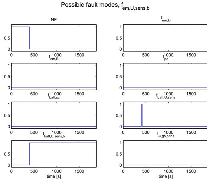
Figure 4.64: Possible fault modes when an offset of 20 V is added to the second sensor signal for the voltage in the battery compared to the true value at 400 seconds.
