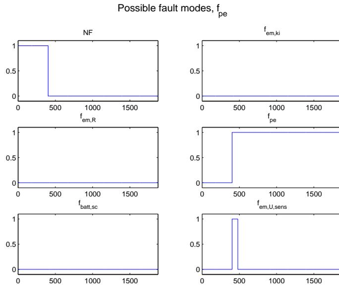
Figure 4.36: Possible fault modes when  $k_{pe}$  is halved at 400 seconds. The fault is detected almost immediately after the fault is induced in the model, while it takes about 80 seconds to achieve full isolability. Test 3 reacts in a few seconds after the test is valid.
