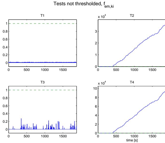
Figure 4.12: Normalized tests before threshold when  $k_i$  is halved at 400 seconds. Tests 2 and 4 reacts fast and there is no doubt that the system is faulty.
