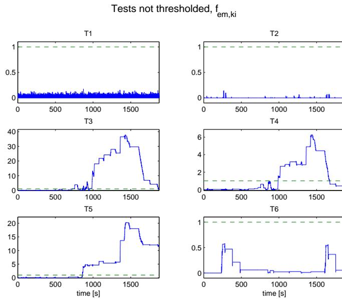
Figure 4.51: Normalized tests before threshold when  $k_i$  is halved. Test 6 should alarm in this fault mode, but there is nothing in the test quantity that indicates this. Therefore it is impossible for the system to decide whether it is a fault in the electric machine or the speed sensor in the gear box that is broken. This is in analogy with the decision structure in Table 4.7.
