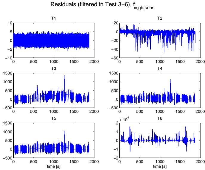
Figure 4.68: The residuals when  $\omega_{gb,sens}$  breaks down at 400 seconds.
