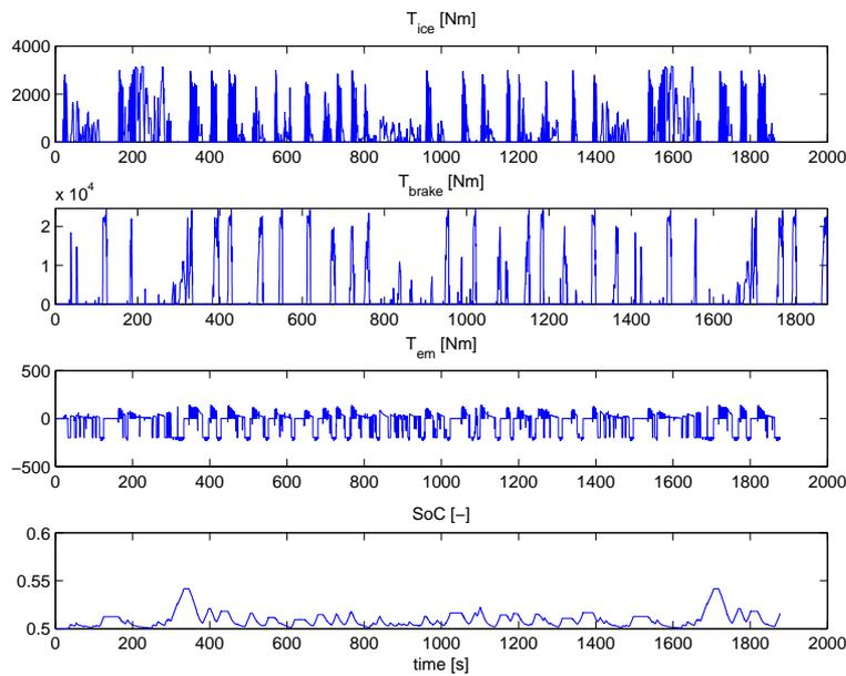
Figure 3.2: Different torques and  $SoC$  when the truck is driving FTP75 with the parameters and models described in this chapter.
