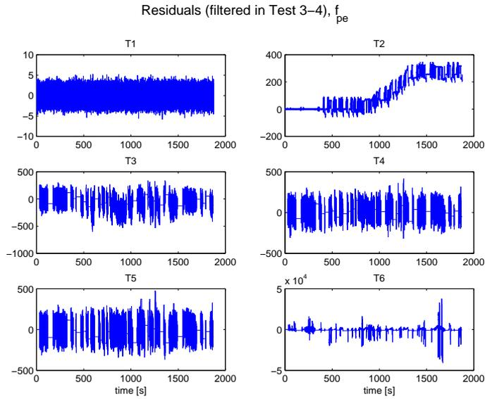
Figure 4.56: The residuals when  $k_{pe}$  is halved at 400 seconds.
