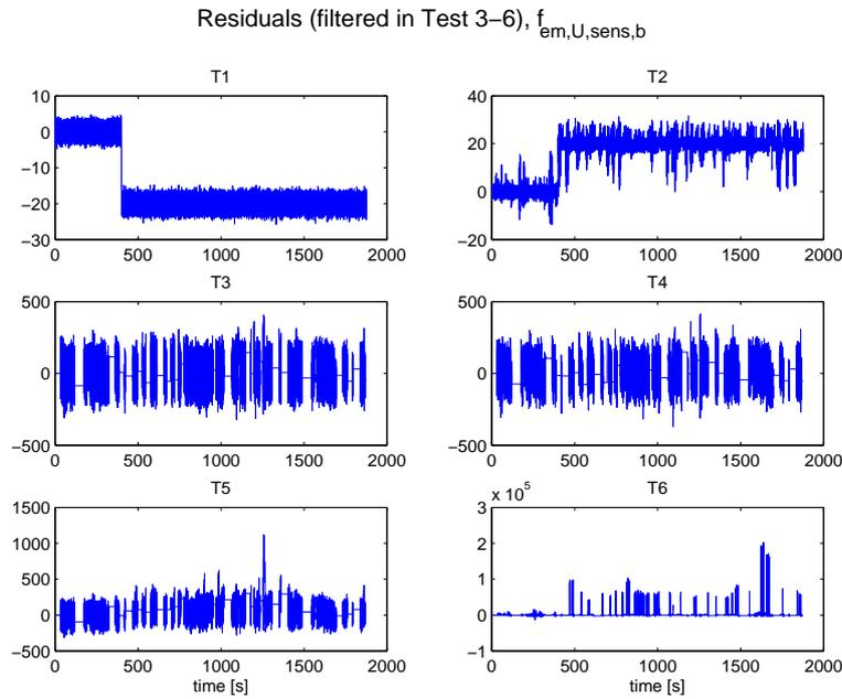
Figure 4.65: The residuals when  $U_{batt,sens,b}$  breaks down at 400 seconds. In the residuals used in test 1, 2 and 6 it is clear that a fault has occurred in the system. In test 5 it is not as easy.
