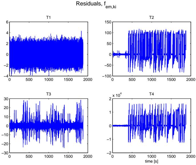
Figure 4.11: The residuals when  $k_i$  is halved at 400 seconds. In this simulation it is clear that the residuals to tests 2 and 4 reacts on the change in the parameter  $k_i$ .
