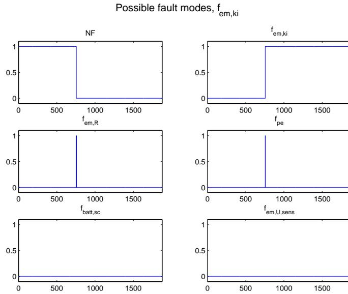
Figure 4.30: The faults detected when  $k_i$  is halved at 400 seconds. The fault is detected and isolated, but it takes about 350 seconds to achieve this. One of the reasons for the long detection time is that the tests 3 and 4 that are supposed to react not are updated for long periods, see Figure 4.29.
