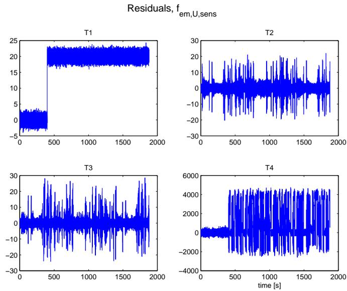
Figure 4.23: The residuals when  $U_{em,sens}$  breaks down at 400 seconds. The residual used in the first test has mean value of approximately 20 V. This is due to that the offset in the sensor has a direct impact on the residual given in equation (4.1).
