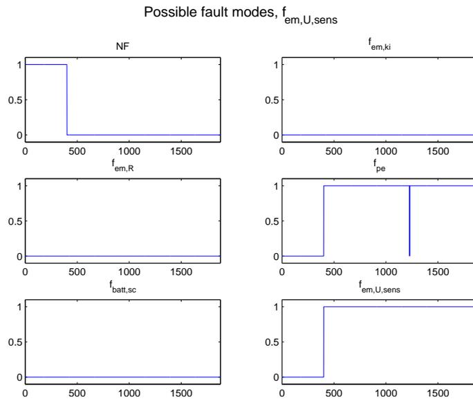
Figure 4.42: Possible fault modes when an offset of 20 V is added to the sensor signal for the voltage in the electric machine at 400 seconds. Also this fault is detected fast, but it takes 350 seconds to achieve isolability.
