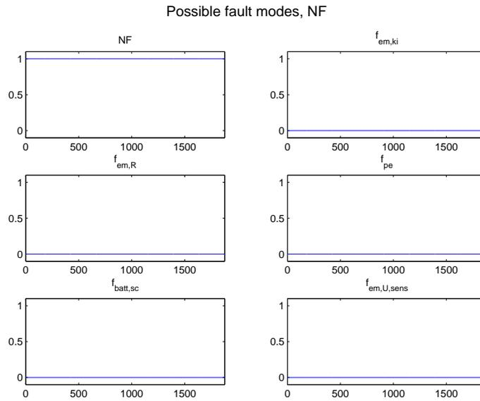
Figure 4.26: No faults are detected in the fault free case.
