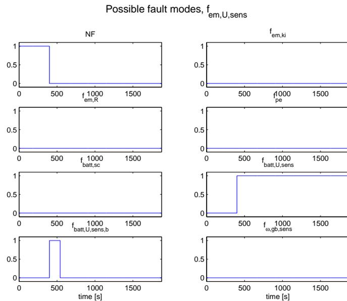
Figure 4.61: Possible fault modes when an offset of 20 V is added to one of the sensor signals for the voltage in the battery compared to the true value at 400 seconds.
