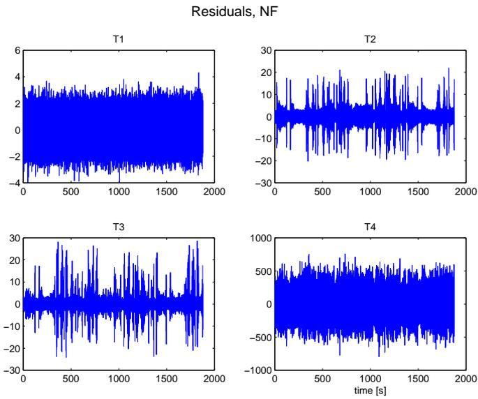
Figure 4.8: The residuals in a fault free case. The magnitude of the residuals in test 2 and 3 varies depending on the operating point of the system. The residuals are largest during transients. One reason for this is that the delays in the model and diagnosis system are not fully synchronized. This results in that different signals are compared from different times in the residual generator.
