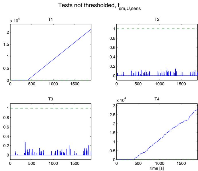
Figure 4.24: Normalized tests before threshold when  $U_{em,sens}$  breaks down at 400 seconds. Both tests 1 and 4 reacts as expected.
