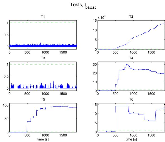
Figure 4.60: Normalized tests before threshold when  $k_{sc}$  is halved at 400 seconds. Tests 4 triggers on the fault during the first period after the fault has occurred. At the end of the simulation the test quantity decreases instead of increase as is preferred. The reason for this could be that the vehicle is driven in a different mode, which not excite the faults in the diagnosis system.
