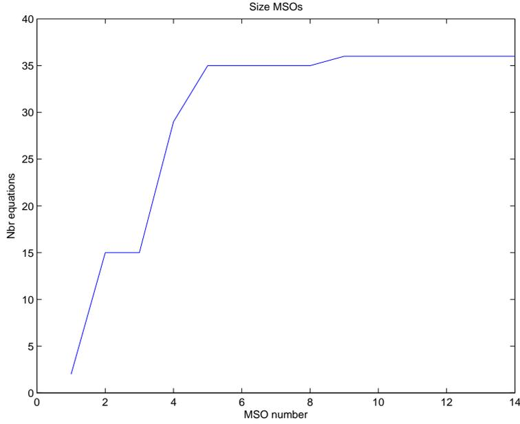
Figure 4.6: The number of equations used in each test for the sensor placement in diagnosis system 3. There is not as many MSOs that include few equations as in the previous diagnosis systems described. There are also less minimal structural overdetermined parts in the system since there are less sensors used.
