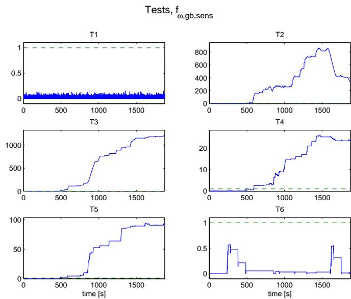
Figure 4.69: Normalized tests before threshold when  $\omega_{gb,sens}$  breaks down at 400 seconds. Tests 2-5 trigger as expected.
