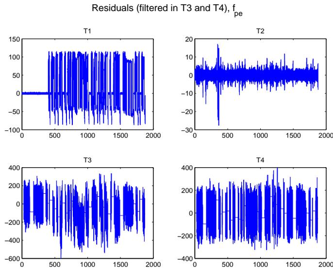
Figure 4.37: The residuals when  $k_{pe}$  is halved at 400 seconds. The large variations in the residual used in test 2 that is shown e.g. at about 350 seconds occurs at gearshifts. At these times the test quantity is not updated and therefore it does not affect the performance of the diagnosis system.
