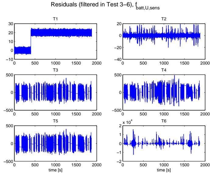
Figure 4.62: The residuals when  $U_{batt,sens,a}$  breaks down at 400 seconds. In the first residual the offset is, as expected, 20 V after the fault is induced.
