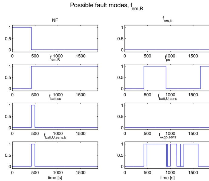
Figure 4.52: Possible fault modes when  $R_{em}$  is halved at 400 seconds. The fault is detected fast, but it is more difficult to isolate the fault.
