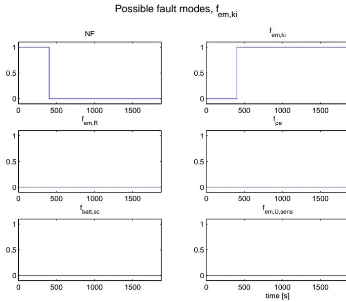
Figure 4.10: Possible fault modes when  $k_i$  is halved at 400 seconds. The fault is detected and isolated in 2 seconds after it occurs.
