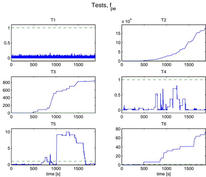
Figure 4.57: Normalized tests before threshold when  $k_{pe}$  is halved at 400 seconds. The most interesting in this figure is that the test quantity in test 4 is larger compared to the fault free case, even though the test shouldn't react according to the design of the test.
