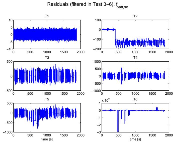
Figure 4.59: The residuals when  $k_{sc}$  is halved at 400 seconds.
