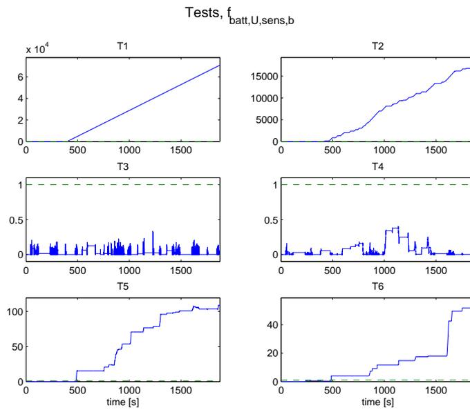
Figure 4.66: Normalized tests before threshold when  $U_{batt,sens,b}$  breaks down at 400 seconds. All tests are working properly.
