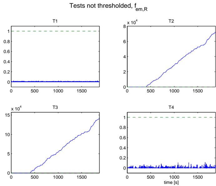
Figure 4.15: Normalized tests before threshold when  $R_{em}$  is halved at 400 seconds. There is no doubt which tests that reacts in this case.
