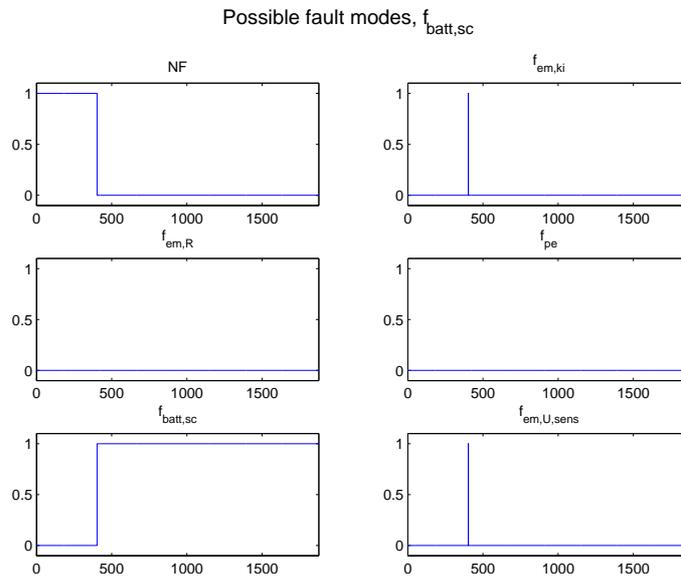
Figure 4.19: Possible fault modes detected when a short circuit in the battery occurs at 400 seconds. Half of the cells are only used after this time. The fault is detected and isolated in 3 seconds.
