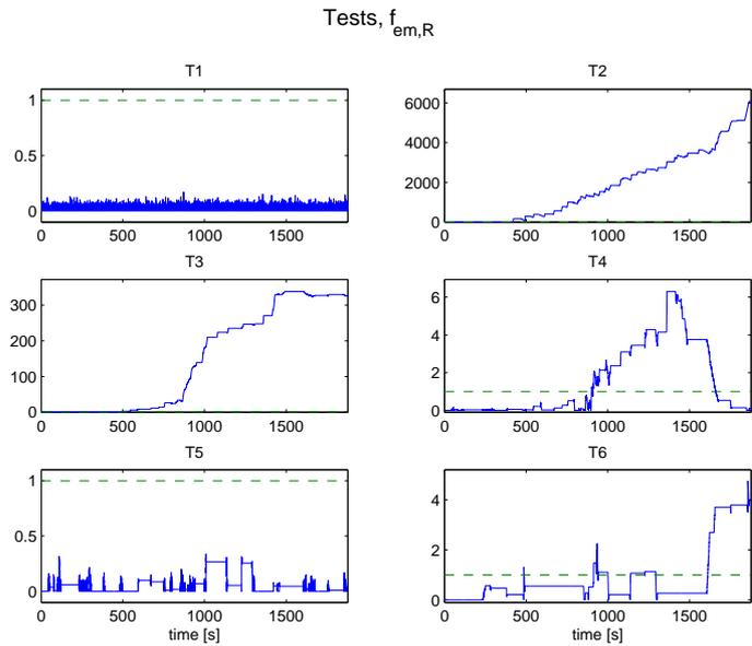
Figure 4.54: Normalized tests before threshold when  $R_{em}$  is halved at 400 seconds. It is mainly test 6 that causes some problems since the test only alarms during short periods.
