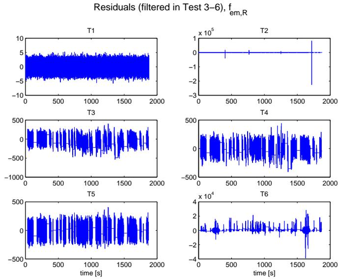
Figure 4.53: The residuals when the resistance in the electric machine is halved at 400 seconds.
