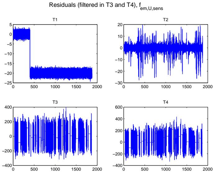
Figure 4.43: The residuals when  $U_{em,sens}$  breaks down at 400 seconds.
