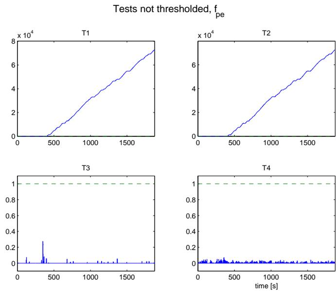
Figure 4.18: Normalized tests before threshold when  $k_{pe}$  is halved at 400 seconds. The magnitudes of the test quantities in the tests that react on the fault are large.
