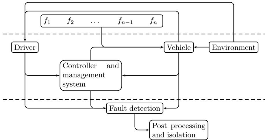
Figure 1.1: The structure of the implemented platform. Above the first horizontal line are the faults induced in the model. Between the lines are the vehicle, driver model, controller and environment. This level includes the information needed to carry out an ordinary simulation. The lowest level includes the diagnosis system.
