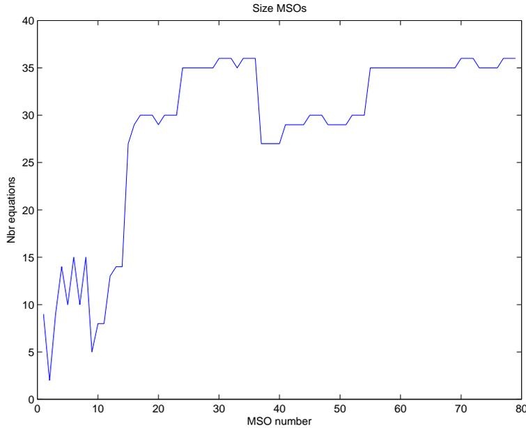
Figure 4.4: The number of equations used in each test for the sensor placement in diagnosis system 2.
