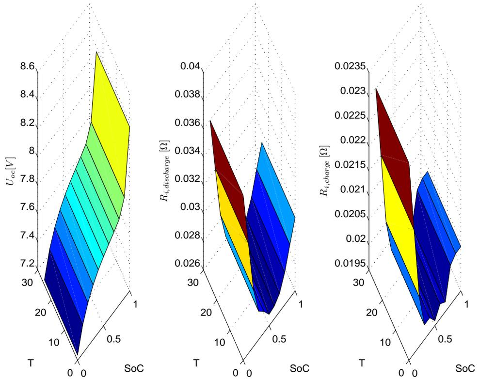
Figure 2.5: The values of the parameters in the model.
