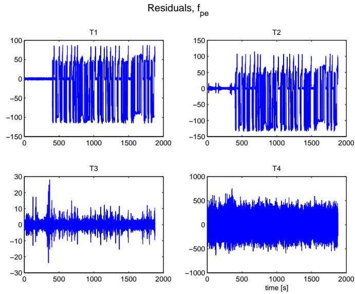
Figure 4.17: The residuals when  $k_{pe}$  is halved at 400 seconds. It is obvious that test 1 and 2 should react, which they also do (see Figure 4.18).
