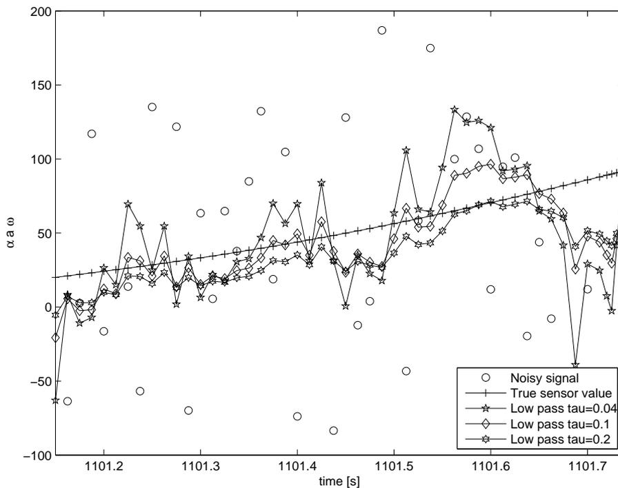
Figure 4.25: Three time constants in the filter of  $\alpha\omega$  is used. Also the unfiltered signal and the sensor signal are included in the figure. As can be seen the filter with low time constant is more noisy than the others, while the filter with high time constant has a time delay during the transient. In the diagnosis systems the time constant is set to 0.1 seconds.
