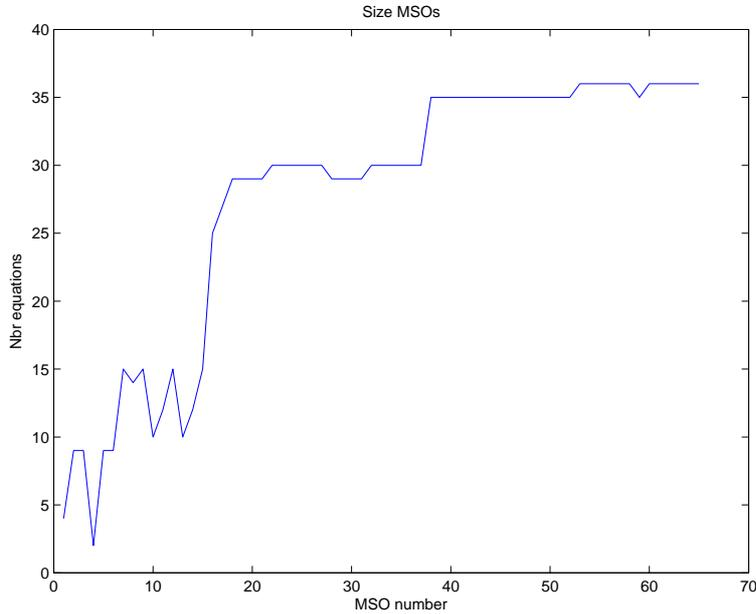
Figure 4.2: The number of equations used in each test for the sensor placement in diagnosis system 1. As seen in the figure there are a few tests based on few equations, but most of the tests are based on a larger part of the entire model that is 48 equations.
