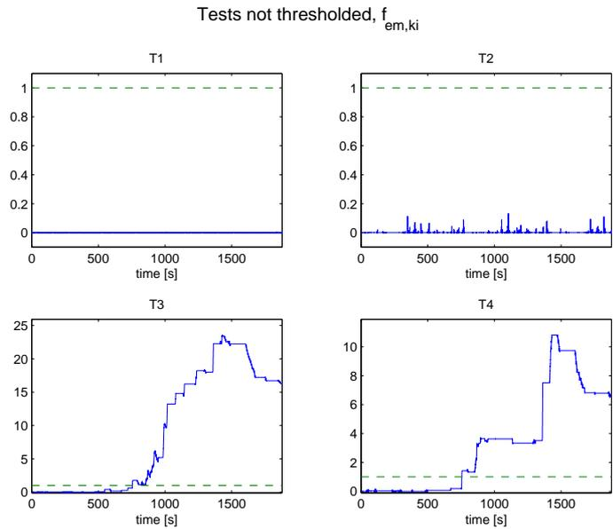
Figure 4.32: Normalized tests before threshold when  $k_i$  is halved at 400 seconds. Both tests that react on this fault have the worrying trend of that the test quantity decreases at the end of the simulation.
