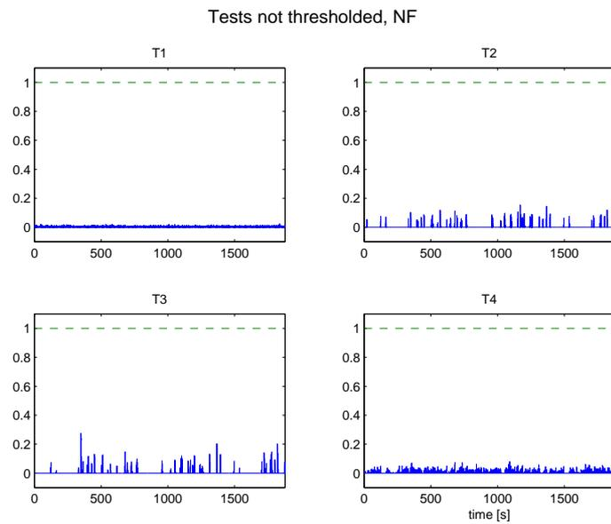
Figure 4.9: Normalized tests before threshold in a fault free case. The test alarms if the test quantity is larger than 1.
