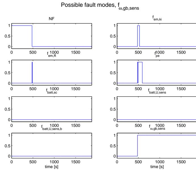
Figure 4.67: Possible fault modes when an offset of  $10 \text{ rad/s}$  is added to the sensor signal for the angular velocity at the outgoing shaft of the gear box compared to the true value at 400 seconds.
