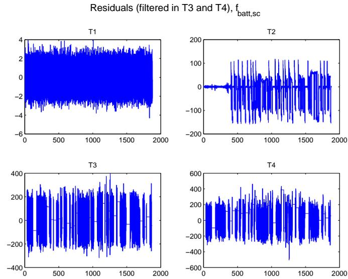
Figure 4.40: The residuals when  $k_{sc}$  is halved at 400 seconds. The residual regarding test 2 clearly changes mode after the fault has occurred. In the residual in test 4 it is more difficult to identify if a fault has occurred or not.
