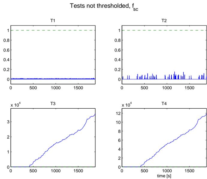
Figure 4.21: Normalized tests before threshold when  $k_{sc}$  is halved at 400 seconds. The tests that are supposed to react, do so with large margins.
