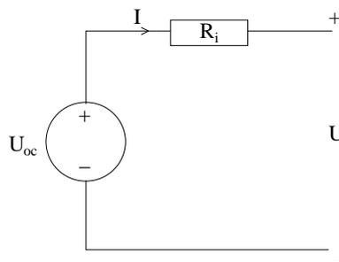
Figure 2.3: The equivalence circuit used in `buffer_simple1` model.
