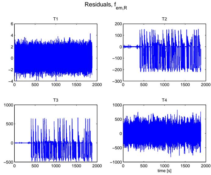
Figure 4.14: The residuals when  $R_{em}$  is halved at 400 seconds. It is clearly shown that the residuals for tests 2 and 3 changes magnitude when the fault is induced in the system.
