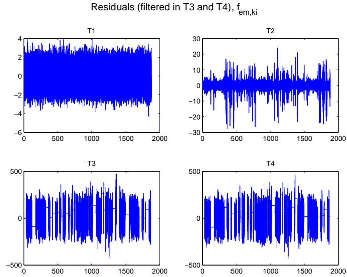
Figure 4.31: The residuals when  $k_i$  is halved at 400 seconds. In tests 3 and 4 there are periods where the residual not is updated. This is when the model used in the diagnosis system is not valid and therefore the residual is not updated.
