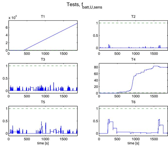
Figure 4.63: Normalized tests before threshold when  $U_{batt,sens}$  breaks down at 400 seconds. Test 1 and 4 trigger as expected from the decision structure.
