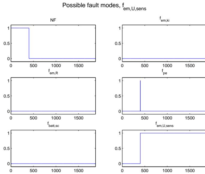
Figure 4.22: The faults detected when an offset of 20 V is added to the sensor signal for the voltage in the electric machine compared to the true value at 400 seconds. The fault is detected in less than one tenth of a second and isolated in 3 seconds.
