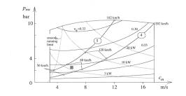
$\begin{array}{l} \mbox{Additionally: Also geometric ratio between gears.} \\ \frac{i_{g,1}}{i_{g,2}} \approx \frac{i_{g,2}}{i_{g,3}} \approx \frac{i_{g,3}}{i_{g,4}} \approx \frac{i_{g,4}}{i_{g,5}} \end{array}$
