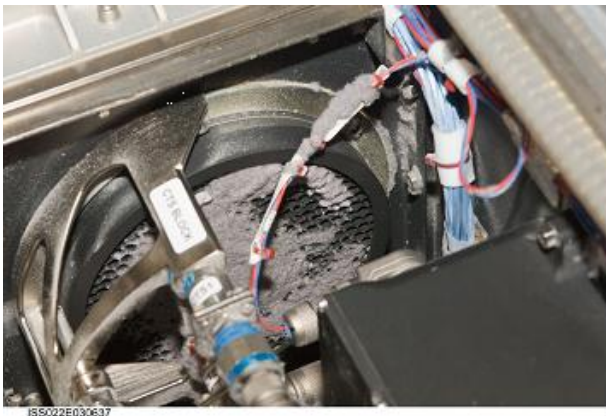
FIGURE 6. Dust Collection in the air loop
