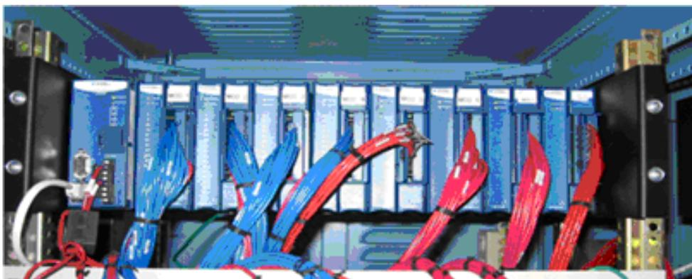
Figure 3.19. Picture of a Compact FieldPoint backplane taken from [17].
