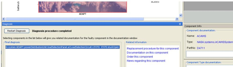
Figure 5.16. Screenshot of the RODON IMBD (Interactive model-based diagnosis) environment. Enough measurements have been inserted and the faulty relay has been isolated. RODON can provide the user with information about the component as depicted in the bottom right of the figure.
