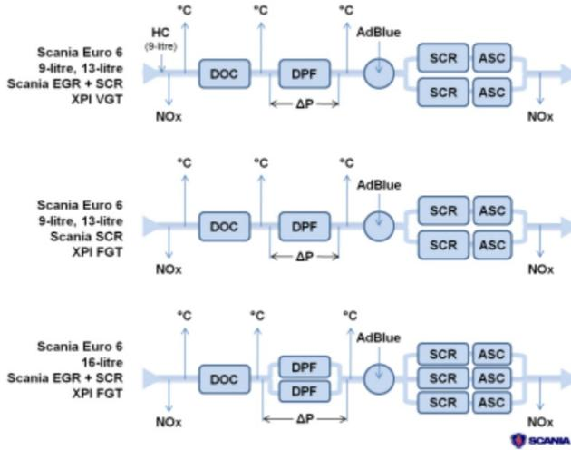
**Figure 4.5:** The exhaust aftertreatment system components that are fitted inside the muffler.  $\text{NO}_x$ -sensors are mounted at the inlet and outlet. The temperature is measured in every step and the pressure drop over the particulate filter is measured to determine its condition. [17]
