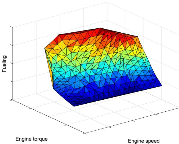
**Figure 4.2:** The surface of triangles generated by the delauney triangulation.
