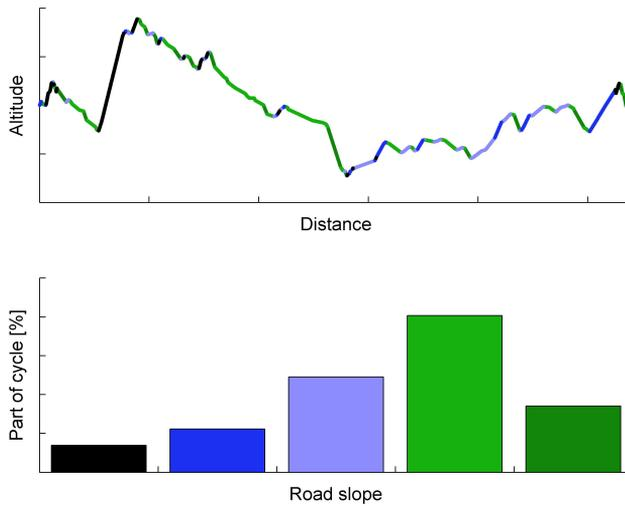
**Figure 3.1:** In VO, parts of the road with similar slope are lumped together. The fuel consumption is then estimated using a method similar to the average operating point method described in section 2.3
