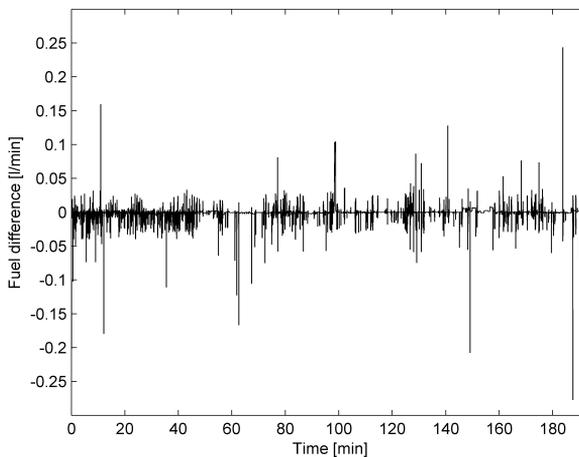
**Figure 4.3:** The difference in instantaneous fuel consumption using two different estimation methods in STARS, using steady state engine maps and compensating for the transient fueling behaviour.
