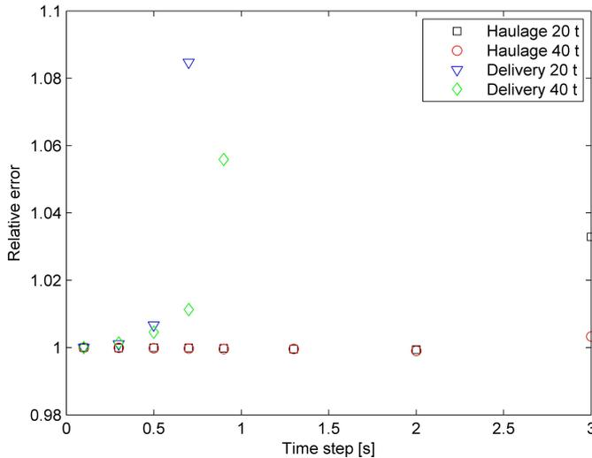
**Figure 5.3:** Plot of the relative error in fuel consumption caused by increasing the time step. Simulations are performed with two different vehicle weights and for two different driving missions, haulage and delivery.
