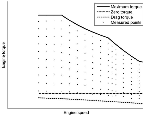
**Figure 4.1:** Example of an engine map (values below a certain speed are hidden).
