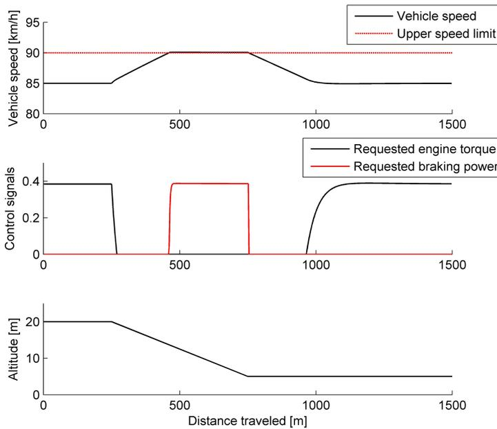
**Figure 5.1:** Illustration of how the cruise controller works. When the vehicle drives downhill and the speed increases, the fueling to the engine stops. Braking only occurs if the upper speed limit is reached.
