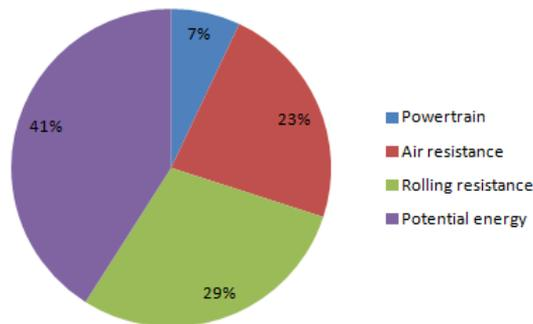
**Figure 2.2:** Illustration of how the energy produced by the engine is distributed. The values are obtained from a simulation of a 40 ton truck on a typical road performed in [5].
