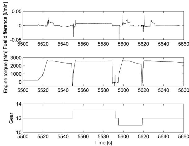
**Figure 4.4:** Engine torque and difference in fuel consumption.
