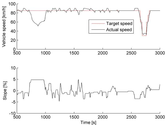
**Figure 3.2:** Example of how a drive cycle in VECTO are converted to a cycle with realistic driving operation.
