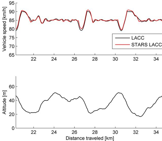
**Figure 7.1:** Comparison of the look-ahead cruise controller (LACC) constructed in this thesis and the one implemented in STARS. The results are obtained from simulations of the road between Södertälje and Norrköping.
