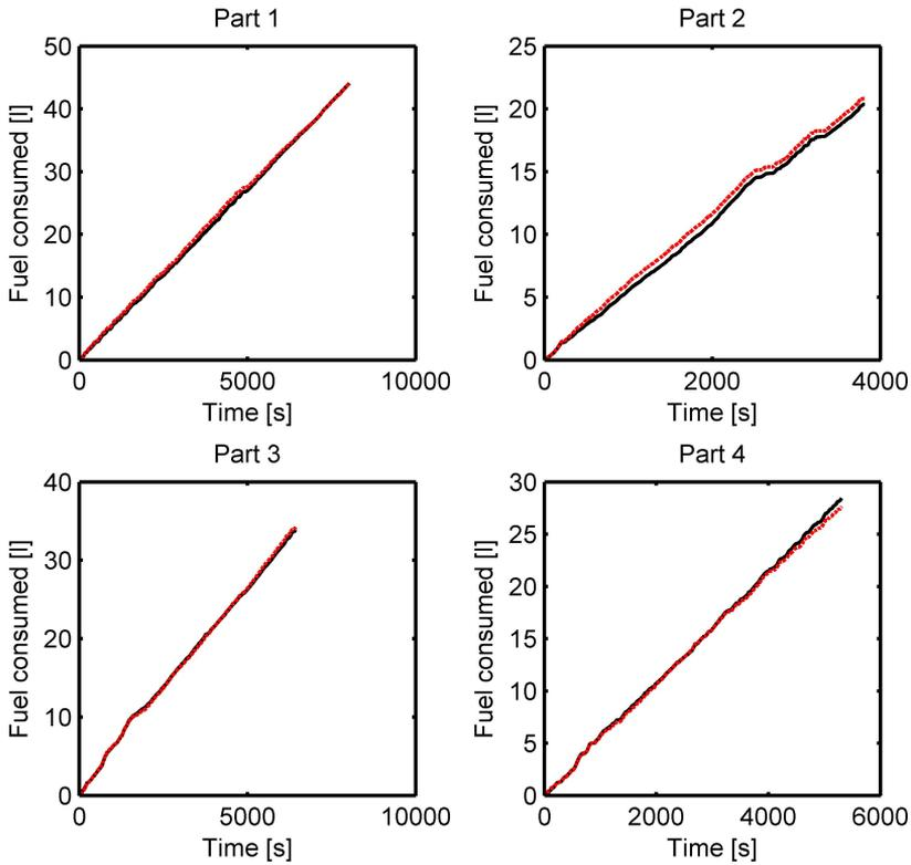
**Figure 6.4:** Cumulative fuel consumption of the different parts of the road between Södertälje and Jönköping. The estimated value (solid line) follows the behavior of the measured value (dotted line) well.
