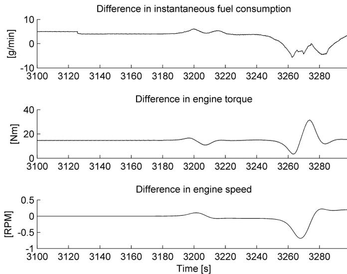
**Figure 6.1:** Difference in engine speed, engine torque and fuel consumption compared to STARS. Positive values is an overestimation compared to STARS.
