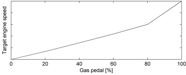
**Figure 5.2:** The gear shifting strategy chooses the gear that gives the engine speed closest to the target speed. The target speed is decided by the gas pedal
