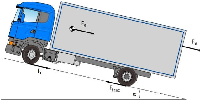
**Figure 4.6:** An illustration of a truck and the forces that affects the translational motion.  $F_{trac}$  is the tractive force,  $F_a$  is the aerodynamic forces,  $F_r$  is the rolling resistance force and  $F_g$  is the gravitational force acting on the vehicle due to road slope.
