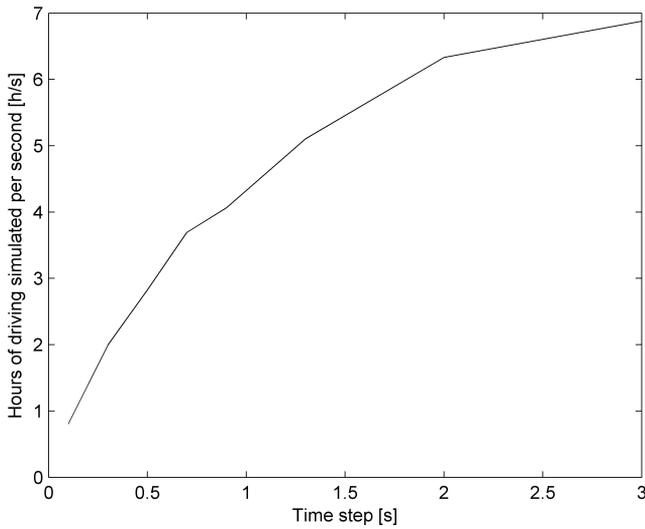
**Figure 5.4:** Plot of how many hours of driving that is simulated in one second for different time step. The values are obtained as the average from the simulations described in figure 5.3.
