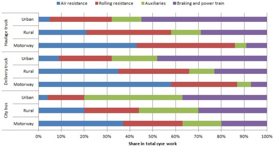
**Figure 2.1:** Distribution of the driving resistances for different vehicle types and driving scenarios [11].
