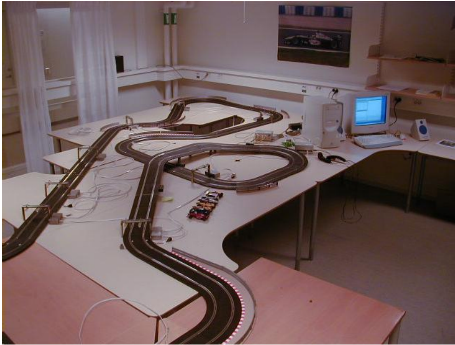
Figure 4.1: Slot car track at Vehicular Systems, including sensors and control system.
