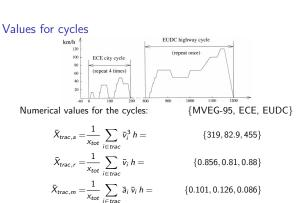
$\bar{E}_{MVEG-95} \approx A_f c_d \, 1.9 \cdot 10^4 + m_v c_r \, 8.4 \cdot 10^2 + m_v \, 10$  kJ/100 kmTasks in Hand-in assignment
