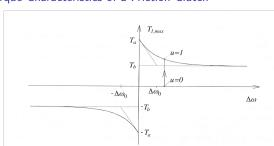
Approximation of the maximum torque in a friction clutch
