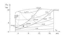
Additionally: Also geometric ratio between gears.  $\frac{i_{g,1}}{i_{g,2}} \approx \frac{i_{g,2}}{i_{g,3}} \approx \frac{i_{g,3}}{i_{g,4}} \approx \frac{i_{g,4}}{i_{g,5}}$
