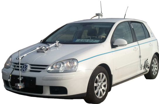
Figure 1: The vehicle-dynamics testbed for studying critical maneuver handling.
